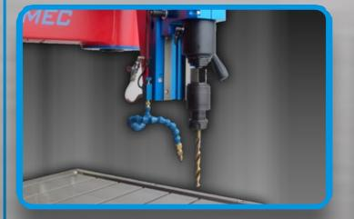
WITH THIS SYSTEM IS POSSIBLE TO ENSURE A CORRECT NEBULIZATION'S TOOL.
